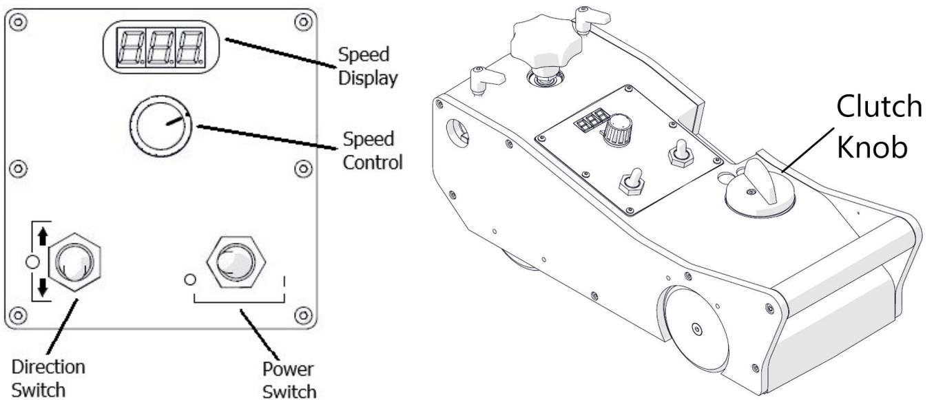
Set the power switch to 'I' to turn on the machine. Then, the display comes on (888) and the display will momentarily show  $U5$ . Next, the travel speed shows. Use the speed knob to set the desired speed. If needed, set the clutch knob to OFF and travel the machine by hand to your starting location.
