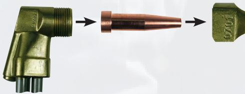
1. Remove the cutting tip and tip nut from the oxy-fuel torch.
