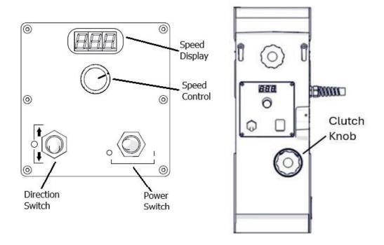
Set the power switch to I' to turn on the machine. Then, the display comes on (8.8.8.) and the display will momentarily show US. Next, the travel speed shows. Use the speed knob to set the desired speed. If needed, set the clutch knob to OFF and travel the machine by hand to your starting location.
